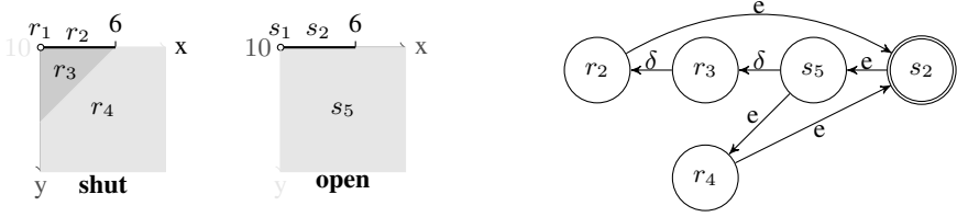
Fig. 5. 0-DBB Abstraction: Partitioning of the Regions and Control Graph of the Abstraction (for simplification the cycle r_1 \leftrightarrow s_1 is left out)
